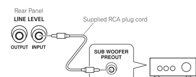
This connection is for an amplifier or receiver equipped with a SUBWOOFER PREOUT terminal. Connect to the LINE LEVEL INPUT terminal on this unit, using the specially provided RCA plug cord.
