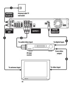
1 Connect RF antenna cables as shown.
