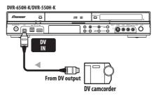
Use a DV cable (not supplied) to connect the DV jack of your DV camcorder to the front panel DV IN jack of this recorder.
