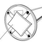
Acoustic control material Apply acoustic control material sheet to the bottom surface of the speaker system stand. Take care not to allow the sheet to come between the small skid-pads and
