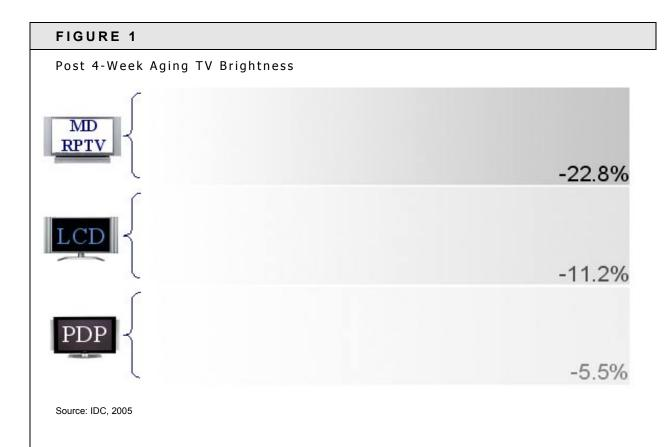
*Test Results* – As illustrated in Figure 1, the plasma TVs that were tested showed a smaller amount of light output decrease, and therefore outperformed all the TV technologies. The post 4-week aging brightness measurement for plasma was -5.5%, whereas the LCD brightness decreased by 11.2%, and microdisplay rear projection TVs declined by 22.8%.
