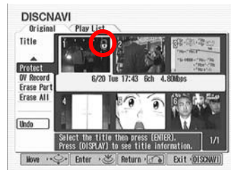
Figure 7-1: protected title (1) has a padlock icon in the upper right corner of the thumbnail.
