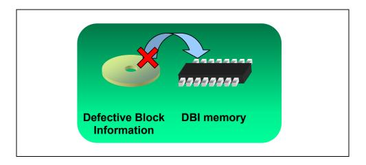
If the drive detects a defective block during read operations, its address and other related information such as defect level are stored in the DBI memory. The same holds true during real-time streaming.
