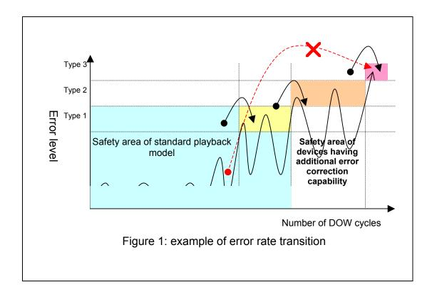
The Mt. Fuji Group has defined a defect transition model that is necessary for real-time recording for RW media. Figure 1 shows that errors detected in a given DVD-RW media sector may increase after many overwrite cycles. When this happens, the error level of such sectors may be changed from a lower level to higher level; it is not allowed to suddenly change from an error level lower than a Type 1 to a Type 3.
