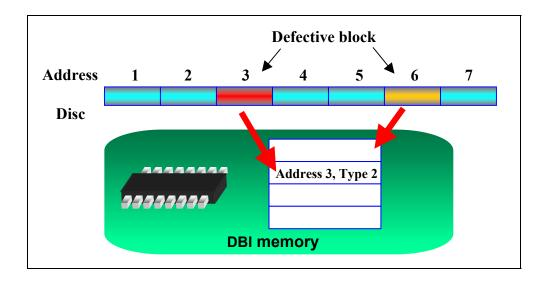
When the Drive detects an overwrite to a defective block during a real-time stream write operation, it is reported to the host. The host is then able to perform a defect management operation after the completion of the real-time streaming operation by referring to the information stored in the DBI memory.
