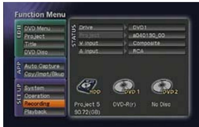
Arrow right to access the **Video/Audio** submenu. Using arrow buttons, select the video encode rate for your production. Changes to the video rate can affect the amount of available recording space. To verify that your recording fits on the disc, monitor the *Remain* information while adjusting the encode rate. Press **Enter** to select an encode rate.
