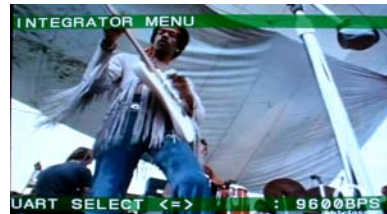
C. Down (V) key then Left or Right keys to set the desired Baud Rate.
