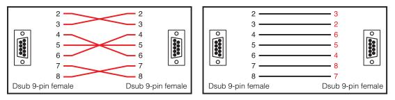
• The following cable has been proved to ensure system operation.
