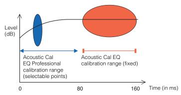
Figure 1 Comparison of microphone data acquisition time periods
