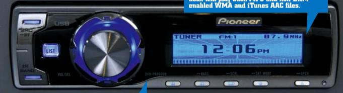
The key cosmetic focus on the deck is the blue OEL (Organic Electro-Luminescent) dot matrix display and the large rotary control. The OEL display has a resolution of 160 x 48 pixels and can display up to three lines of text, each with an impressive 16 characters per line. That's twice what most competing products offer. Pioneer calls the control the Rotary Commander.
