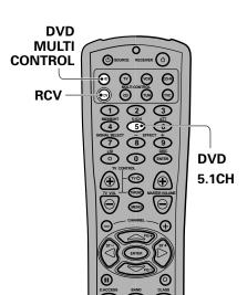
There are two ways to switch on DVD 5.1 CH mode. With the remote control press the DVD/LD MULTI CONTROL button. Then press the RCV button and number button 5 (DVD 5.1CH). On the main unit simply press the DVD button.
