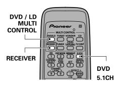
There are two ways to switch on DVD 5.1 CH mode. With the remote control press the DVD/LD MULTI CONTROL button. Then press the RECEIVER button and number button 4 (DVD 5.1CH). On the main unit simply press the DVD 5.1CH button.
