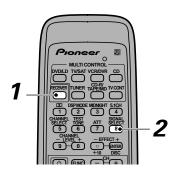
Each press switches between ANALOG and DIGITAL signal selection.
