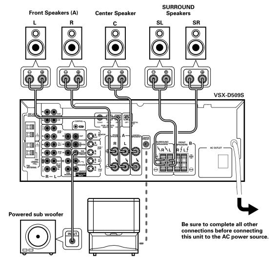
When using the speaker on your TV as the center speaker, connect the CENTER PREOUT jack on this unit to the audio input jack on your TV. In this case, the center speaker shown is unnecessary.
