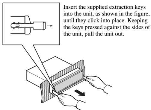
Insert the supplied extraction keys into the unit, as shown in the figure, until they click into place. Keeping the keys pressed against the sides of the unit, pull the unit out.
