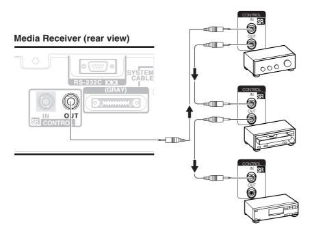
The control cables (not supplied) are mono sound cables with mini plugs (no resistance).
