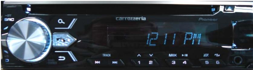
2. Press the M.C. (multi-control) to display the "INITIAL" menu and then press again to enter.
