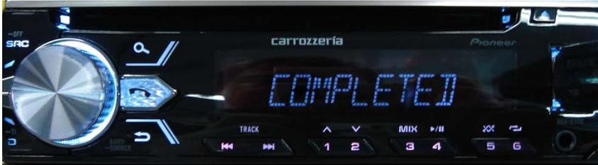
11. The product will reboot automatically after the update is finished. Do not touch anything even when the screen is blacked out. After it has finished rebooting, the screen will return to the initial screen.
