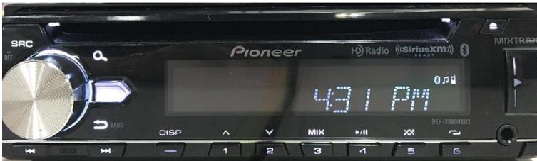
3. Press M.C. (multi-control) dial to display the "Initial" menu, then press to confirm.
