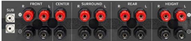
Figure 2: Rear panel of AVR; the height speaker connections are at right.
